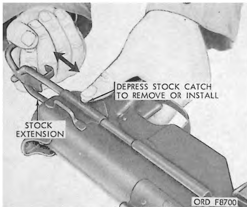
Figure 11. Remove/install gun stock extension.
